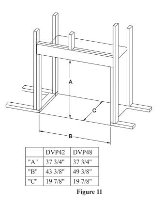
Attention: If a base or mantel is not used and the appliance is installed directly on carpeting, tile or other combustible material other than wood flooring, it shall be installed on a metal or wood panel extending the full width and depth of the appliance. The vertical dimension in Figure 11 must be adjusted when a metal or wood panel is placed beneath the appliance.
